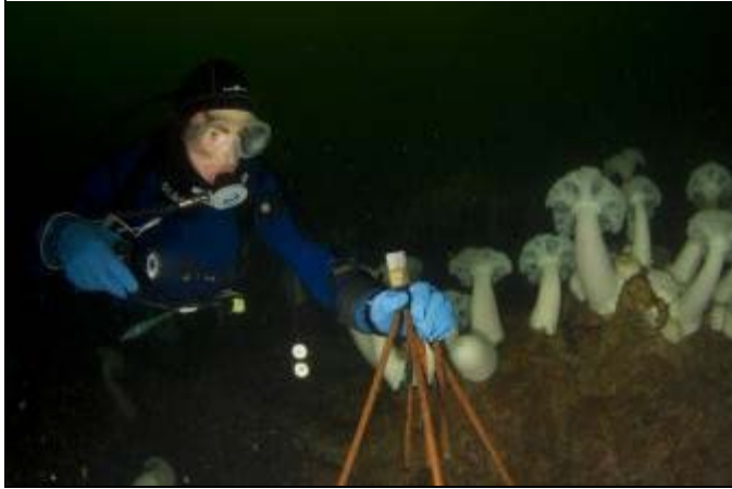
Tavish Campbell helps install the King Island hydrophone Photo Credit: Ian McAllister
