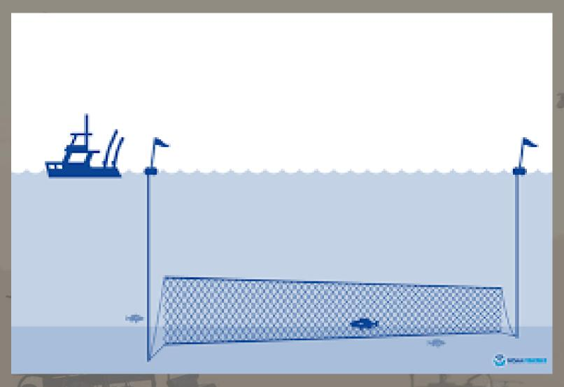
Commercial fishing method using vertical panels of netting to catch fish as they swim into the net.
